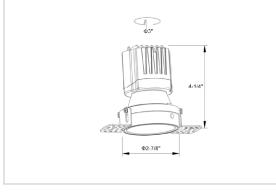
Light Distribution Wide flood LED Type COB LED Light Source Osram SOLERIQ S 19 Start Time Instant Driver Stand Alone (included) **Operating Position** Non - Swiveling Type On-Off / Triac / 0-10 V Dimmina Construction Round Mounting Type Recessed Single Head Heads **Body Material** Aluminium Die cast Finish Black 4" Height Diameter 3-1/2' Cut Out 3" Darklight Technology Black, Silver Optics
