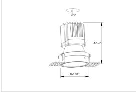
CRI >90 Beam Angle 60° Light Distribution Wide flood LED Type COB LED Light Source Osram SOLERIQ S 19 Start Time Instant Driver Stand Alone (included) **Operating Position** Non - Swiveling Type On-Off / Triac / 0-10 V Dimmina Construction Round Mounting Type Recessed Single Head Heads **Body Material** Aluminium Die cast Finish Black 4" Height Diameter 3-1/2'
