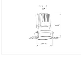
2700K CCT CRI >90 Beam Angle 15° Light Distribution Spot COB LED Type LED Light Source Osram SOLERIQ S 19 Start Time Instant Driver Stand Alone (included) **Operating Position** Non - Swiveling Type On-Off / Triac / 0-10 V Dimmina Construction Round Mounting Type Recessed Single Head Heads **Body Material** Aluminium Die cast Finish Black 4" Height 6-1/2" Diameter Cut Out 3"
