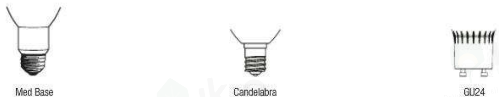
Figure 39. Screw based CFL bases(left and center) and 2 pin base of GU24
